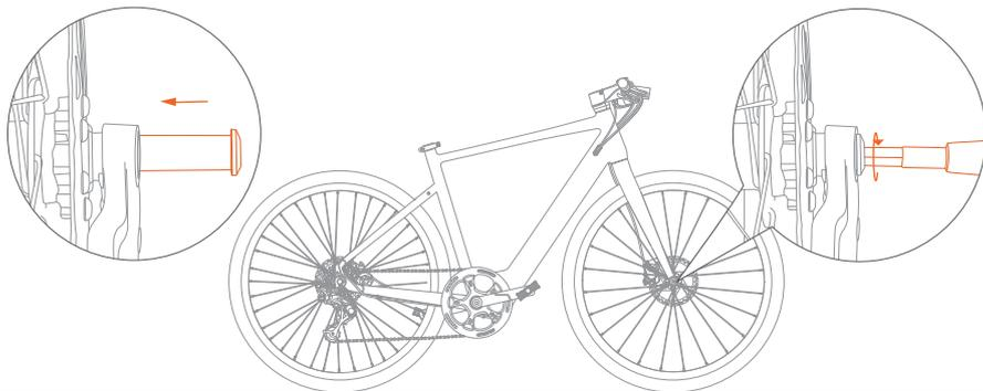
③ Put the shaft through the front wheel and tighten it clockwise with a three-prong wrench to complete the installation for front wheel.
