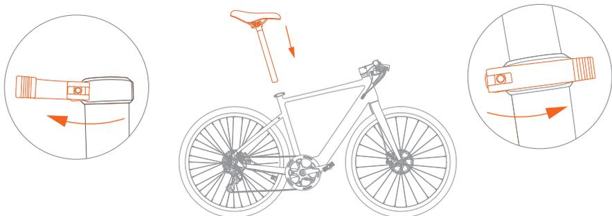
① Open the seat clamp, insert the seatpost.
