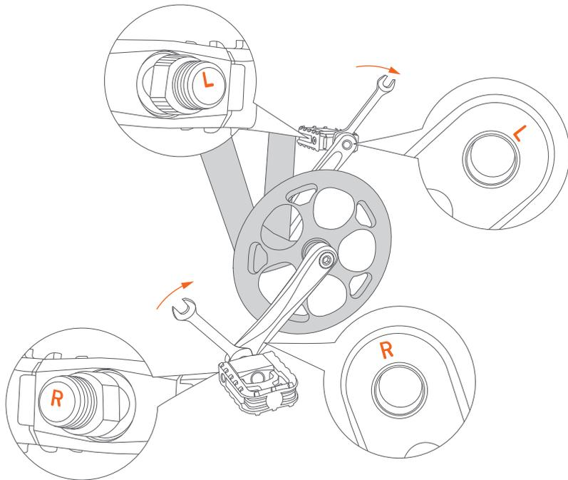
Use the open spanner of the tools bag, screw the pedal shaft into the threaded hole and tighten it in the direction of the arrow.
