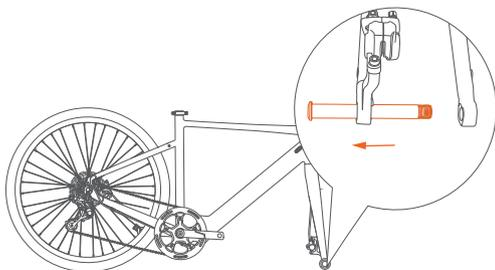
① Remove the front brake spacer and unscrew the shaft on the front fork.
