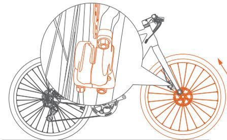
② Lift the front part of the bike, align the front wheel and insert the front fork sleeve ring.
