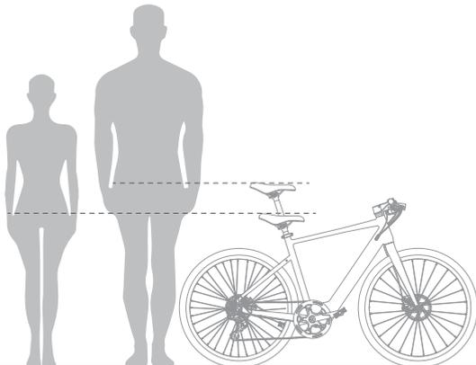
② Adjust the seatpost to suitable height, the recommended height is when the saddle is level with the user's pelvis when standing naturally. The height of the adjustment can NOT exceed the safety line.
