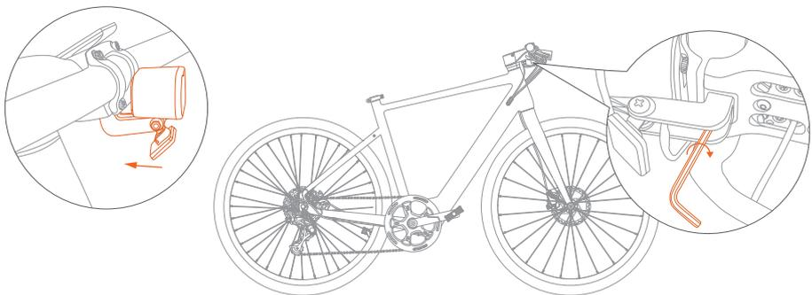
Align the headlight screw hole with the bottom hole of the handlebar, insert the screw and tighten it.
