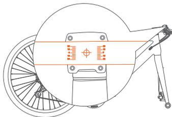
② Align the handlebar scale to the front of the bike.
