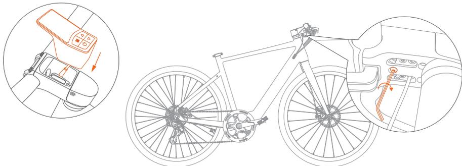
Place the meter in the groove of the handlebar. Use the hexagonal tool to tighten the screw to fastening the meter on the handlebar.
