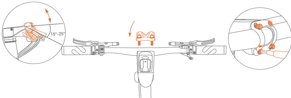
③ Cover the riser cover, use a three-fork wrench to lock the screws, then rotate the handlebar and adjust the brake angle to 15~25° downward parallel to the ground, and then tighten the screw
